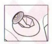
If the Control Stick is held at an angled position (as shown in the picture on the left) when the power is turned ON, this position will be set as neutral. This will cause games using the Control Stick to operate incorrectly.
